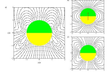
FIG. 3: (Color online) Flow streamlines around a moving Janus particle in the laboratory frame. a) The cap forms an isotherm with  $t_k$  as in (3). b) Dipolar approximation with  $t_1$  only. c) Thin-cap limit, with  $t_{2k} = 0$ .
