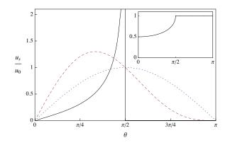
FIG. 2: (Color online) Quasi-slip velocity  $u_s(\theta)$  as a function of the polar angle  $\theta$ . For comparison, we plot the infinite series (4) (solid line), the dipolar approximation (series truncated at n = 1, dotted line) and the quadrupolar approximation (series truncated at n = 2, dashed line). Inset: surface temperature  $[T(a, \theta) - T_0]/\Delta T$  as a function of  $\theta$ .
