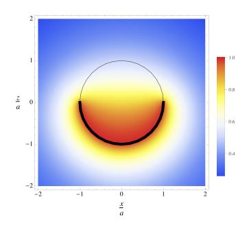
FIG. 1: (Color online) Map of the reduced temperature  $(T-T_0)/\Delta T$  in the (xOz) plane, inside and outside the metalcoated colloid. The thick line represents the metal layer, where the temperature is at its maximum. It then decreases monotonically to the bulk value.
