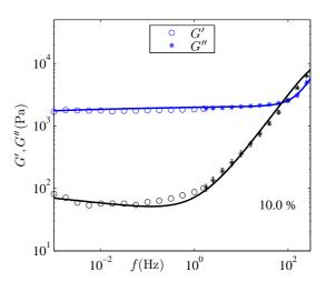
Fig. 6: Rheology of the 10% acrylamide gel. Rheometrical (open circles) and AFM (stars, with standard deviations shown) experimental data. Solid lines are the best model fits.
