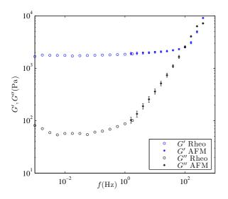
Fig. 2: Superposition of rheometrical (open circles) and AFM measurements (stars, with standard deviations shown). The acrylamide content is 10% in this case.  $T = 25^{\circ}$ C.
