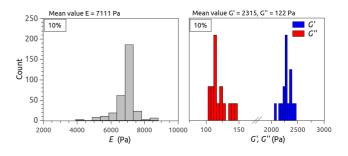
Fig. 1: Histograms showing the 10% gel rheological properties: elastic modulus (E) and dynamic moduli G' and G'' at 1 Hz.  $E = 7111 \text{ Pa} \pm 34 \text{ Pa}, G'(1Hz) = 2315 \text{ Pa} \pm 25 \text{ Pa}.$  Note that  $E \sim 3 G'$ .
