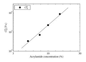
Fig. 8: Evolution of gel modulus  $G_{\rm N}^0$  vs. concentration. The slope of the power law exponent corresponds to  $3.0\pm0.3$ .
