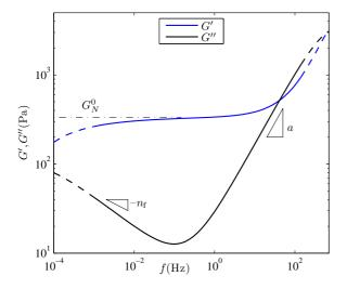
Fig. 3: Significance of the model parameters:  $G_{\rm N}^0$  (plateau modulus),  $n_{\rm f}$  (slope of G'' at low frequencies), and a = b (slopes of G' and G'' at high frequencies).  $\omega \sim 1/\lambda_{\rm max}$  corresponds to the intersection of G' and G'' occuring for very low frequencies (not shown).  $G_1$  corresponds to a higher plateau modulus in G' for  $\omega \sim 1/\lambda_1$ , but is well above our data.
