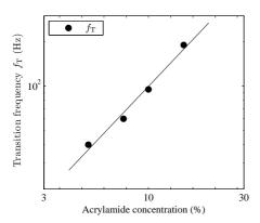
Fig. 9: Evolution of transition frequency  $f_{\rm T}$  vs. concentration. The power law exponent is  $1.6 \pm 0.1$ .
