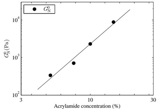
FIG. 4: Evolution of gel moduli  $G_N^0$  vs. concentration. The slope of the power law exponent corresponds to  $3.0 \pm 0.3$ .
