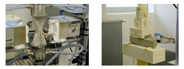
Figure 11: Zoom on the active parts of the tensile test device (left) and of the 4-point bending test device (right) in the room temperature configuration.
