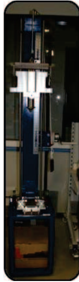
Figure 6: Impact testing instrument MTT
