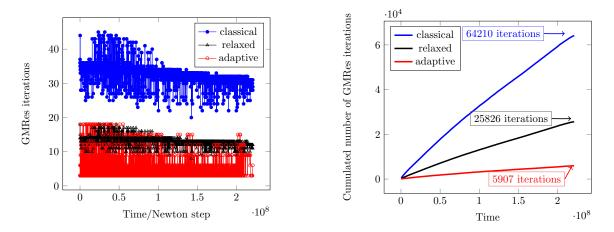
Figure 11: GMRes iterations at each time and Newton step (left) and cumulated number of GMRes iterations as a function of time (right) for the test case of Section 5.3. Average number of GMRes iterations per time and Newton iteration step: 33 iterations (classical), 13 iterations (relaxed), 6 iterations (adaptive). Average number of GMRes iterations per time step: 150 iterations (classical), 61 iterations (relaxed), 14 iterations (adaptive)
