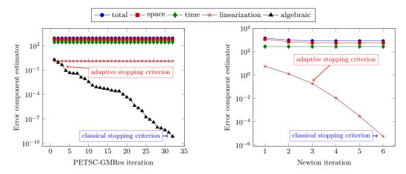
Figure 2: Evolution of the spatial, temporal, linearization, and algebraic error estimators (4.20) for a fixed mesh at time  $1.04 \cdot 10^6$ s, as a function of GMRes iterations on the first Newton iteration (left) and of Newton iterations (right)
