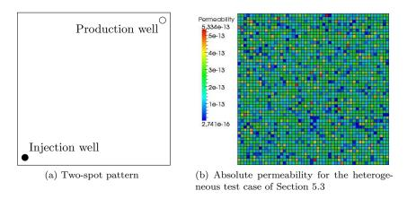
Figure 1: Configuration for the numerical test cases
