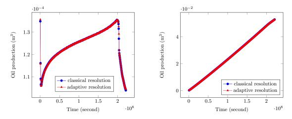
Figure 4: Instantaneous (left) and cumulated oil production (right) during the simulation, classical resolution vs. adaptive resolution for the test case of Section 5.2
