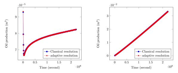
Figure 8: Rate (left) and cumulated rate (right) of oil production during the simulation, classical resolution vs. adaptive resolution for the test case of Section 5.3
