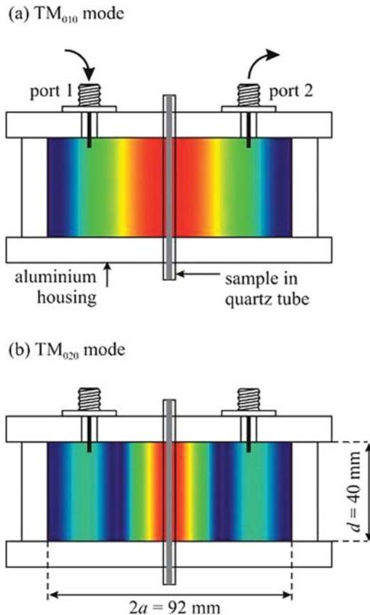
FIG. 2. Schematic diagram of the aluminium host cavity, also showing the magnitude of the electric field in (a) the  $TM_{010}$  mode, and (b) the  $TM_{020}$  mode. In both cases, the field is parallel to the axis of the cylinder. Samples are introduced along the axis, contained in a thin-walled quartz capillary of inner diameter 2 mm. For such small capillaries, we may assume that the applied field is uniform for both modes.
