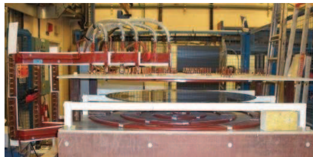
Fig. 4. Induction heating device coils, disc and bus-bar.
