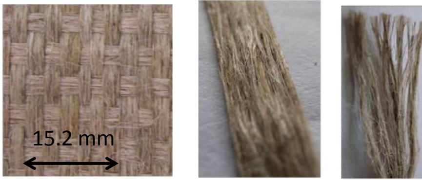
Figure 1: Architecture of reinforcement 1 at the scales of the fabric and the tow.
