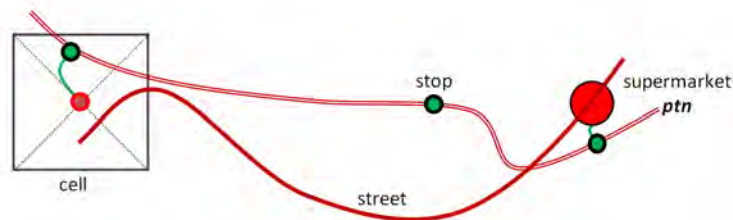
Figure 31: Depiction of the rule set for accessibility; green lines correspond to pedestrian access by using the street network.
