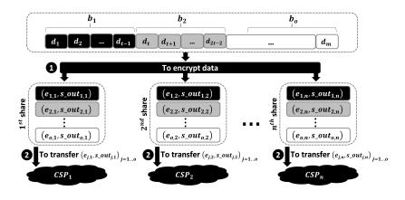
FIG. 3 – Data sharing process in Scheme-I
