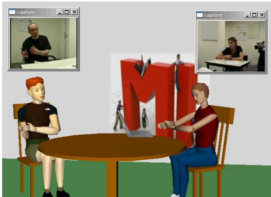
Fig. 5. Real-time motion capture using a single camera for each user and virtual rendering. Demonstration videos are available from http://MyBlog3D.com .
