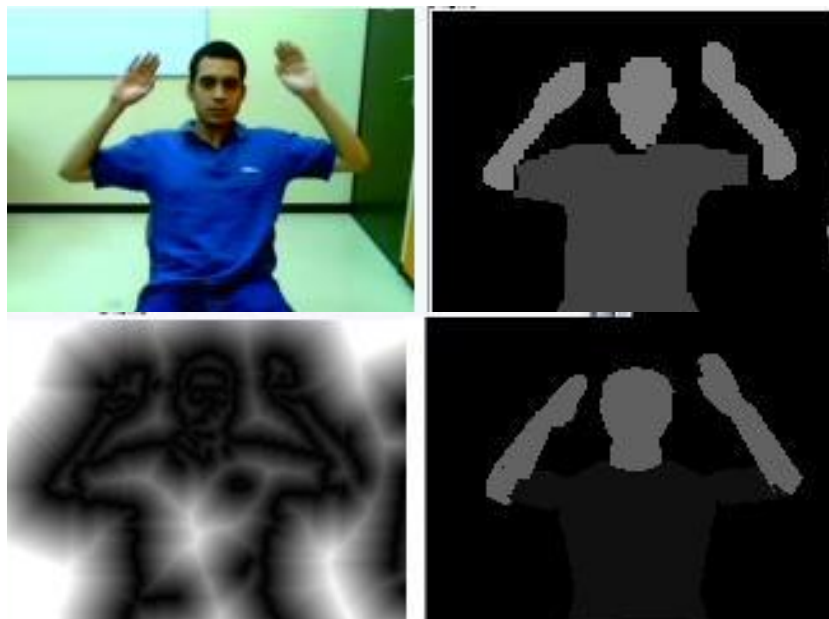
Fig. 4. The captured image, the color-segmented image, map of distance to image edges in the foreground mask and finally the projection of the 3D human body model in the optimal matching pose.
