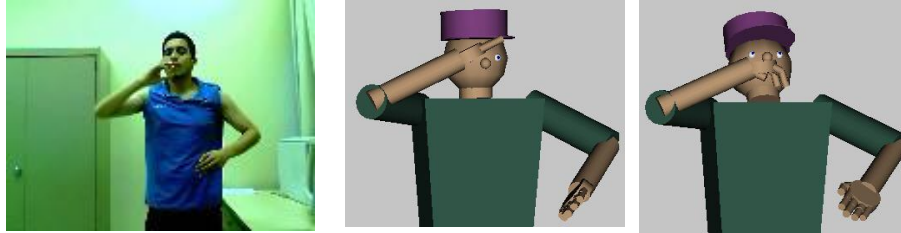
Fig. 11. Augmenting motion capture with gesture models. Left: Input image. Middle: Tracking without gesture model: the hand shape is not captured to meet real-time computation constraints. Right: The gesture model augments the motion capture with fingers movements.
