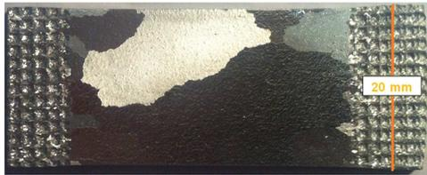
Figure 1: Revealed microstructure after recrystallization
