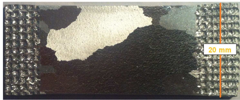
Figure 1: Revealed microstructure after recrystallization
