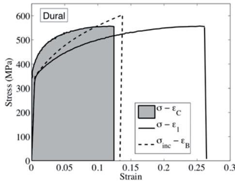
Figure 1: Local (within the localization zone) stress-strain diagrams for the studied material (dural). Measured  $\sigma$  vs.  $\varepsilon_{11}$  relation (solid line); Identified  $\sigma_{\text{inc}}$  vs.  $\varepsilon_C$  relation (dashed line); Identified cohesive zone response (solid line with grey surface)
