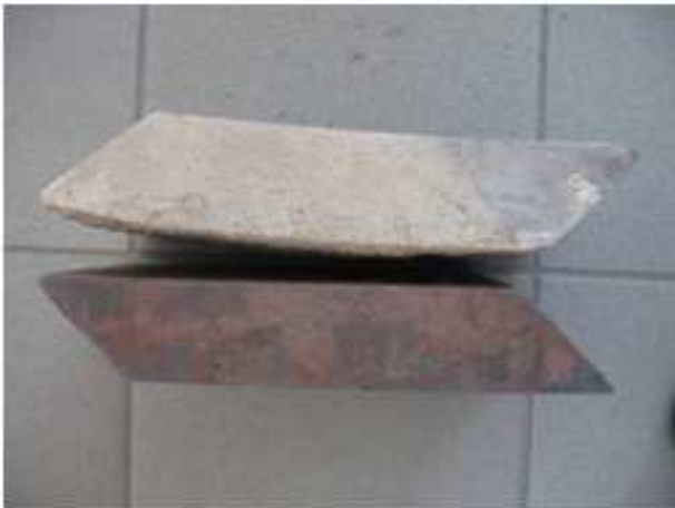
(b) New (bottom) and worn (top) tile after use
