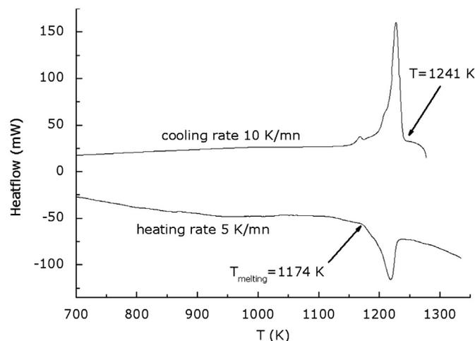
Fig. 6. DSC measurement of the  $\text{PbFe}_3\text{O}(\text{PO}_4)_3$  powder.
