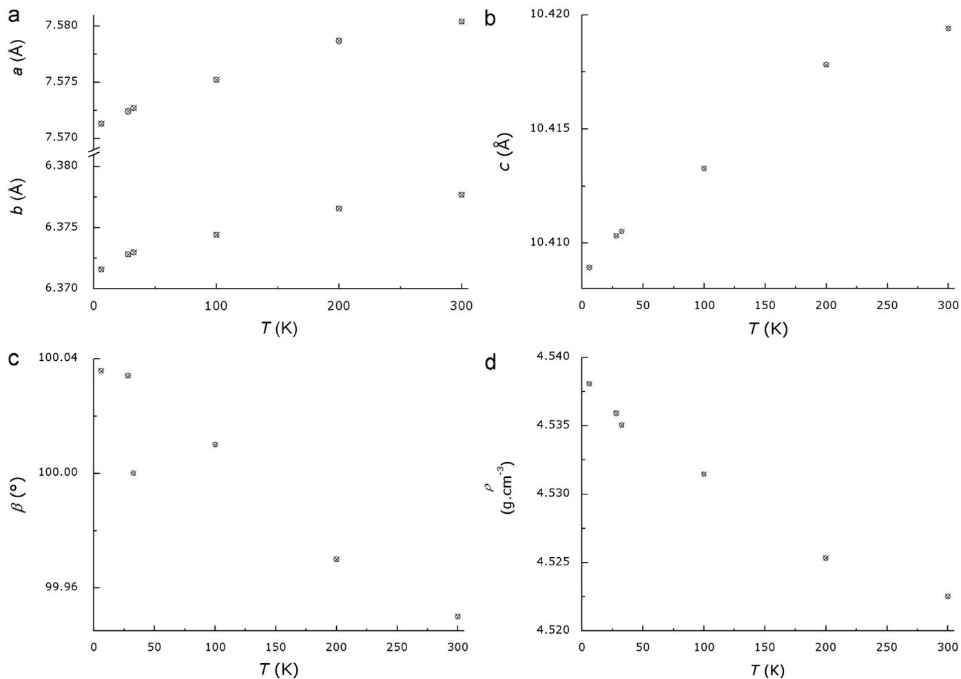
**Fig. 5.** (a)–(c) Thermal dependence of the  $\text{PbFe}_3\text{O}(\text{PO}_4)_3$  lattice parameters; (d) thermal dependence of the  $\text{PbFe}_3\text{O}(\text{PO}_4)_3$  calculated volumic mass.
