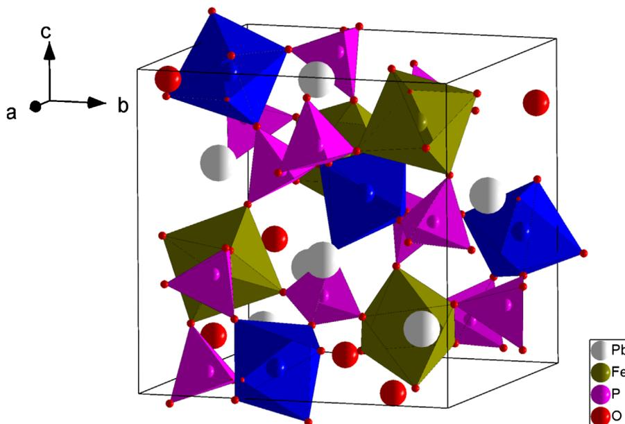
**Fig.1.** Drawing of the  $\text{Pb}_{1.5}\text{Fe}_2(\text{PO}_4)_3$  basic unit cell which shows two crystallographically nonequivalent  $\text{Fe}^{3+}$  cations (brown and blue colors). (For interpretation of the references to color in this figure caption, the reader is referred to the web version of this article.)
