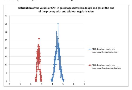
**Figure 11**: distribution of the values of  $CNR_g$  between dough and gas at the end of the proving with and without regularisation. The values were obtained from 1000 Monte-Carlo simulations including the uncertainty on the signal references and on the signal.
