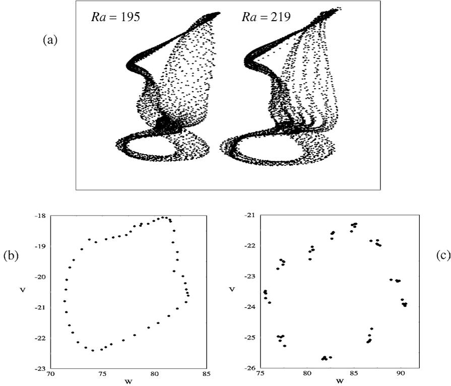
**Figure 9.** (a) Bidimensional projections of the torus in the phase-space and Poincaré's sections obtained at  $Ra = 193$ ; (b) in the quasiperiodic regime and at  $Ra = 219$ ; (c) in a frequency locked state for which the lowest frequency of the system is 11 times smaller than the fundamental one,  $f_1$  (remark the 11 spots in (c)).
