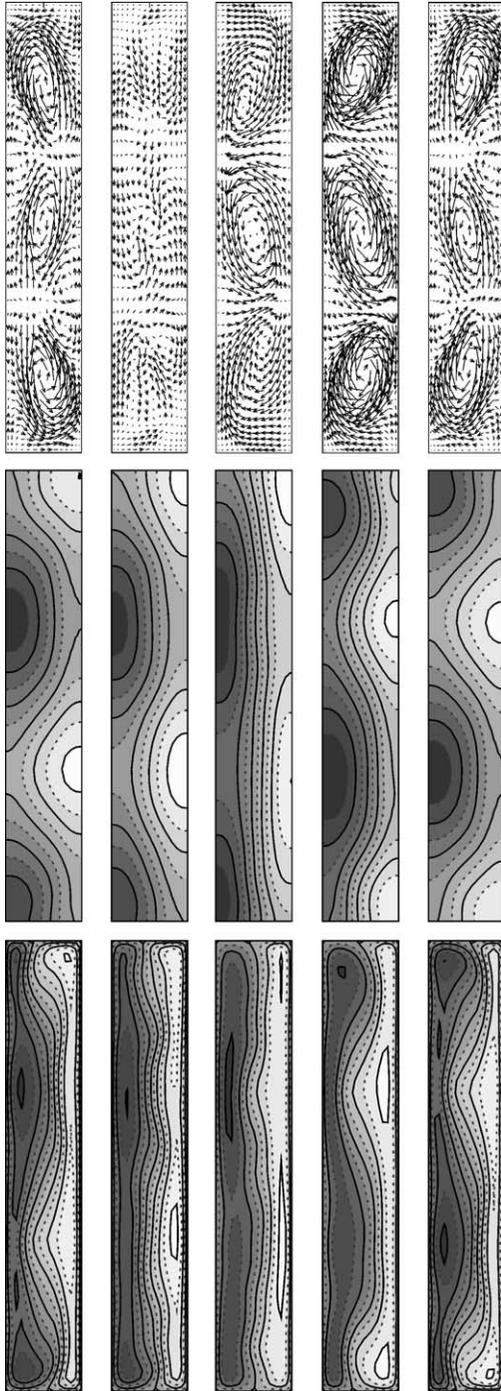
**Figure 4.** From above to below, snapshots of the vector field, isothermals and isovalues of the  $z$ -velocity at the plane  $z = 1.1A_z^{-1}$  (near the center of the enclosure) along a semiperiod of the oscillation. The results correspond to  $Ra = 62.5$  and the fundamental frequency is  $f_1 = 3.65\nu/h^2$ .
