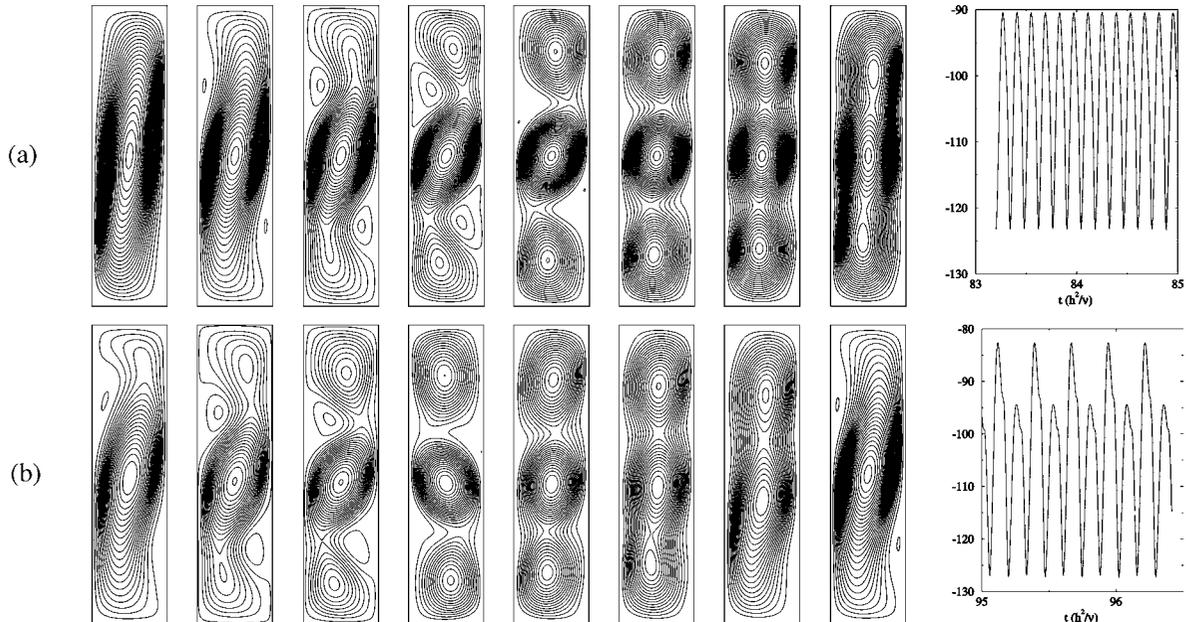
**Figure 3.** Streamfunctions of the two-dimensional flow: (a) Snapshots along a period of motion at  $Ra = 90$  and (b) at  $Ra = 100$  along the period associated to the fundamental frequency,  $1/f_1^{(2D)}$ . The time signal of the streamfunction at  $x = 0.12$  and the central section  $z = A_z^{-1}$  is shown in both cases.
