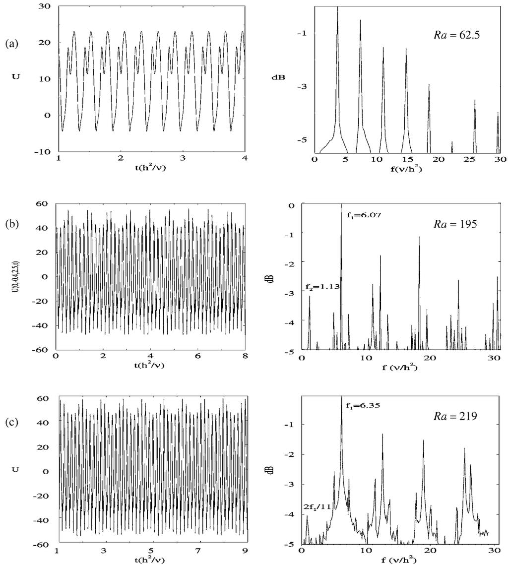
**Figure 8.** Time signal of the  $x$ -velocity obtained at  $x/h = -0.09$ ,  $y = -0.80A_z^{-1}$  and  $z = 1.26A_z^{-1}$  (with  $x \in [-1, 1]$ ,  $y \in [-A_y^{-1}, A_y^{-1}]$  and  $z \in [0, 2A_z^{-1}]$ ) and its power spectra for (a)  $Ra = 62.5$ , (b)  $Ra = 195$  and (c)  $Ra = 219$ .
