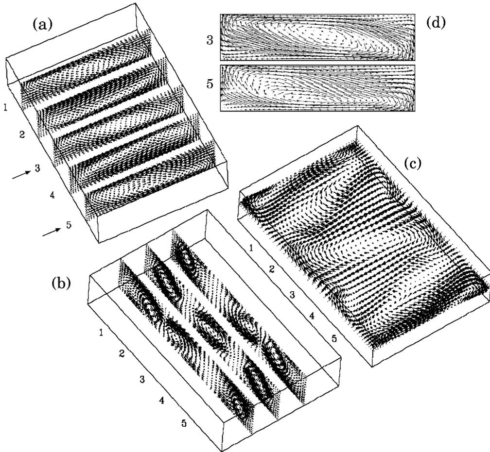
**Figure 6.** Snapshots of the flow at  $Ra = 195$  at an instant of maximum intensity of the perturbative flow in the  $(x, y)$ -plane. The snapshots correspond to an instant of time separated from those in *figure 5* by a quarter of period of the fundamental cycle. For (a), (b), (c) and (d) see the caption of *figure 5*.
