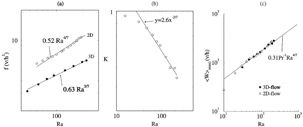
**Figure 7.** (a) Fundamental frequency of the 3D and the 2D flow versus  $Ra$ ; (b) and (c) show respectively the mean temperature  $z$ -gradient at the core  $K$  and the maximum value of the mean  $z$ -velocity of the flow,  $\langle W_{\max} \rangle$ , versus  $Ra$ .
