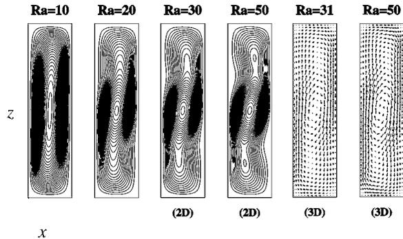
**Figure 2.** From left to right, the first three figures correspond to the streamfunction of the 2D stationary flow. The vector field plots correspond to the 3D oscillatory flow at  $Ra = 30$  and  $Ra = 47$  at approximately the center of the enclosure ( $y = 0.05$ ).
