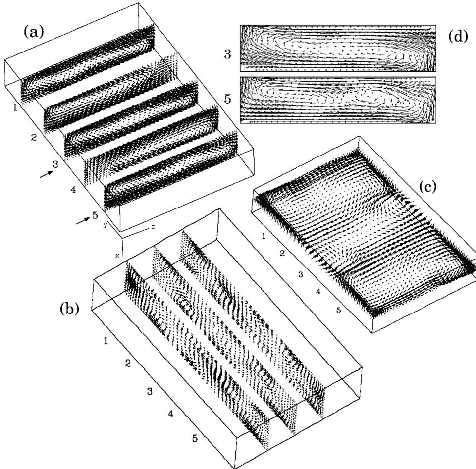
**Figure 5.** Snapshots of the flow at  $Ra = 195$  at an instant of minimum intensity of the perturbative flow in the  $(x, y)$ -plane. (a), (b) and (c) show cuts of the vector field at respectively  $y = cte$ ,  $z = cte$  and  $x = cte$  planes. (d) Magnification of the vector field in the  $y = cte$  planes labeled in (a) by 3 and 5.
