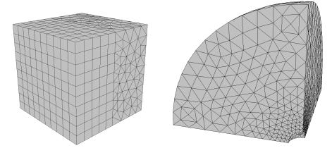
(e) Hybrid grid made of 3432 tetrahedra, 100 (f) Tetrahedral grid of a truncated sphere pyramids and 500 hexahedra. made of 6623 cells.
