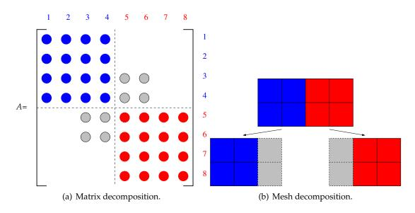
Figure 6: Example of matrix and mesh decomposition on two processors with overlaps construction.
