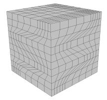
(c) Kershaw-type grid made of 1000 cells.
