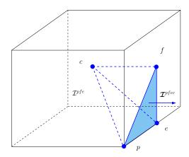
Figure 1: Definition of the iota cell  $\mathcal{I}^{pfe}$  and the outward normal vector  $\mathcal{I}^{pfec}$  related to point p, face f and edge e in the hexahedral cell c.
