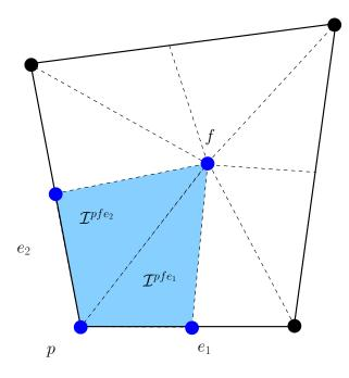
Figure 2: Generic quadrilateral face, f, related to the hexahedral cell  $\omega_c$ . The sub-face,  $\partial \omega_{pc}^{f}$ , related to point p and face f is obtained by gathering the triangular faces corresponding to the iotas  $\mathcal{I}^{pfe_1}$  and  $\mathcal{I}^{pfe_2}$ .
