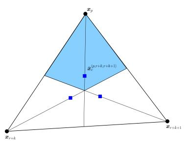
Figure 5: Triangular face (p,r+k,r+k+1) related to the tetrahedron displayed in Figure 4. The sub-face related to point *p* has been colored in blue. The three degrees of freedom related to the sub-face temperatures are plotted by means of blue squares.
