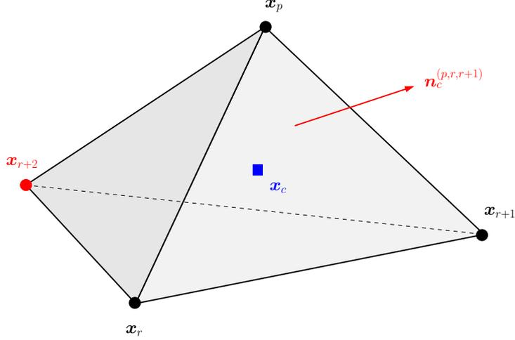
Figure 4: Generic tetrahedron with vertices  $(\mathbf{x}_p, \mathbf{x}_r, \mathbf{x}_{r+1}, \mathbf{x}_{r+2})$  and centroid  $\mathbf{x}_c = \frac{1}{4}(\mathbf{x}_p + \mathbf{x}_r + \mathbf{x}_{r+1} + \mathbf{x}_{r+2})$ .
