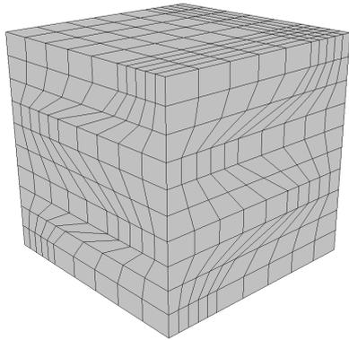
(c) Kershaw-type grid made of 1000 cells.
