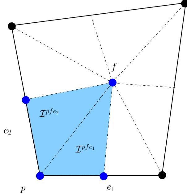
Figure 2: Generic quadrilateral face,  $f$ , related to the hexahedral cell  $\omega_c$ . The sub-face,  $\partial\omega_{pc}^f$ , related to point  $p$  and face  $f$  is obtained by gathering the triangular faces corresponding to the iotas  $\mathcal{I}^{pfe_1}$  and  $\mathcal{I}^{pfe_2}$ .
