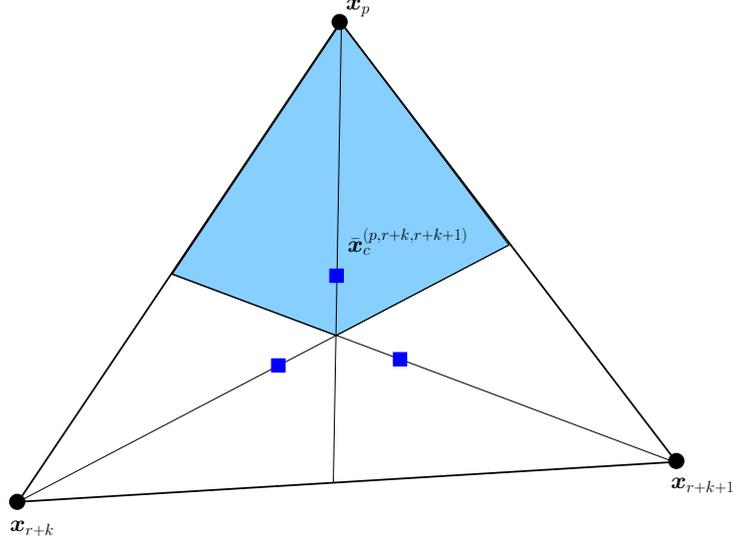
Figure 5: Triangular face  $(p, r+k, r+k+1)$  related to the tetrahedron displayed in Figure 4. The sub-face related to point  $p$  has been colored in blue. The three degrees of freedom related to the sub-face temperatures are plotted by means of blue squares.
