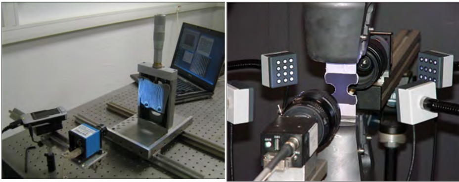
Fig.1. Fringe generation in the case (a) of projected fringes (courtesy of EMSE) (b) of the grid method (courtesy of Arts et Métiers ParisTech)
