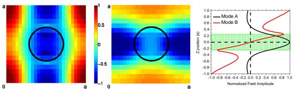
FIGURE 4: MAPPING OF MODE A (LEFT) AND MODE B (CENTER) OVER ONE PERIOD AND  $E_{\rm X}$  FIELD AMPLITUDE IN CROSS SECTION FOR THOSE TWO MODES (RIGHT. MODES A AND B ARE REPRESENTED BY A BLACK AND A RED LINE, RESPECTIVELY). ON THE MAPPINGS, THE HOLE IS DEPICTED BY A BLACK CIRCLE WHILE FOR THE CROSS SECTION VIEW, THE MEMBRANE CORRESPOND TO THE GREEN DASHED AREA. THE PARAMETERS OF THE MEMRBANE ARE FF=0.15, D=a/2 AND K=0.
