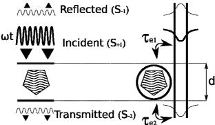
FIGURE 1: LEFT: SCHEMATIC VIEW OF THE ABSORBING THIN FILM RESONATOR STUDIED IN THE FRAME OF THE TDCMT. RIGHT: SAME MODEL TRANSLATED IN TERMS OF MICRORESONATORS COUPLED TO A WAVEGUIDE AS DEPICTED IN [5]. NO SPECIFIC ASSUMPTION IS MADE ABOUT THE SYMMETRY OF THE MODE.
