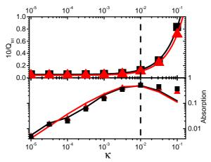
FIGURE 5: 10 /  $Q_{TOT}$  (TOP) AND ABSORPTION (BOTTOM) VARIATIONS VERSUS EXTINCTION COEFFICIENT FOR MODE A (IN BLACK) AND B (IN RED), D=A/2 AND ff=0.15. THE VALUES (SQUARE FOR MODE A, TRIANGLE FOR MODE B) REPORTED ARE FITTED (LINES) BY THE THEORETICAL MODELS DERIVED FROM (7) FOR Q AND FROM (8) FOR THE ABSORPTION. THE DASHED LINE REPRESENTS THE K VALUE SELECTED FOR THE REST OF THE STUDY (CRITICAL COUPLING CONDITIONS)
