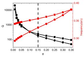
FIGURE 6 : QUALITY FACTOR (IN BLACK) AND FREQUENCY (IN RED) OF THE MODES VERSUS FILLING FACTOR IN AIR FOR D=A/2. MODE A IS REPRESENTED BY SQUARES AND MODE B BY DOTS. THE DASHED LINE CORRESPONDS TO THE PARAMETERS CHOSEN FOR THE STUDY
