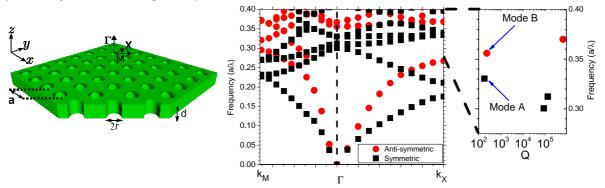
FIGURE 3: LEFT: SCHEMATIC VIEW OF THE 2D PHC MEMBRANE WITH ITS CORRESPONDING PARAMETERS. CENTER: BAND DIAGRAM OF THIS NON ABSORBING MEMBRANE WITH D=A/2 AND FF =0.15 AND FOR BOTH SYMMETRIC (OR EVEN) (BLACK SYMBOLS) AND ANTI-SYMMETRIC (OR ODD) (RED SYMBOLS) MODES. RIGHT: FREQUENCY VERSUS Q FACTOR OF THE MODES IN  $\Gamma$  ZOOMED IN THE FREQUENCY RANGE OF INTEREST.
