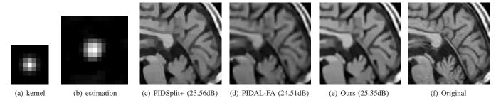
Fig. 10. Results of different methods on Brain image corrupted by a Gaussian blur and Poisson noise with peak intensity 600.
