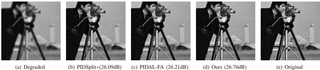
Fig. 9. Results of different methods on Cameraman image corrupted by the Uniform blur and Poisson noise with peak intensity 600.
