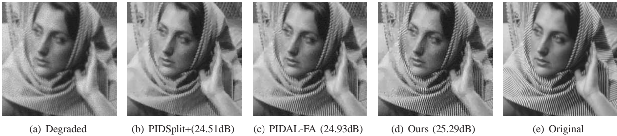
Fig. 7. Results of different methods on Barbara image corrupted by the Gaussian blur and Poisson noise with peak intensity 600.
