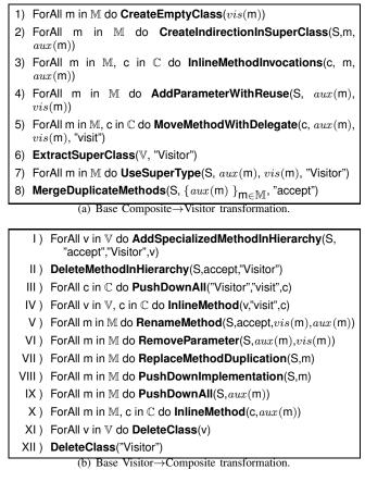
Figure 3. Base Algorithms for reversible transformation from Composite to Visitor.
