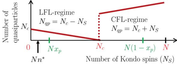
FIG. 3 (color online). Number of quasiparticles as a function of  $N_S$  for fixed  $N_c$ . A transition is expected at  $N_S = N_c$ , when  $x_p < 1/2$ . For realistic (i.e., small) Kondo coupling, only a small part of the conduction electrons is involved in the Kondo screening of the LFL regime, resulting in an intermediate third regime  $Nn^* < N_S < N_c$ .
