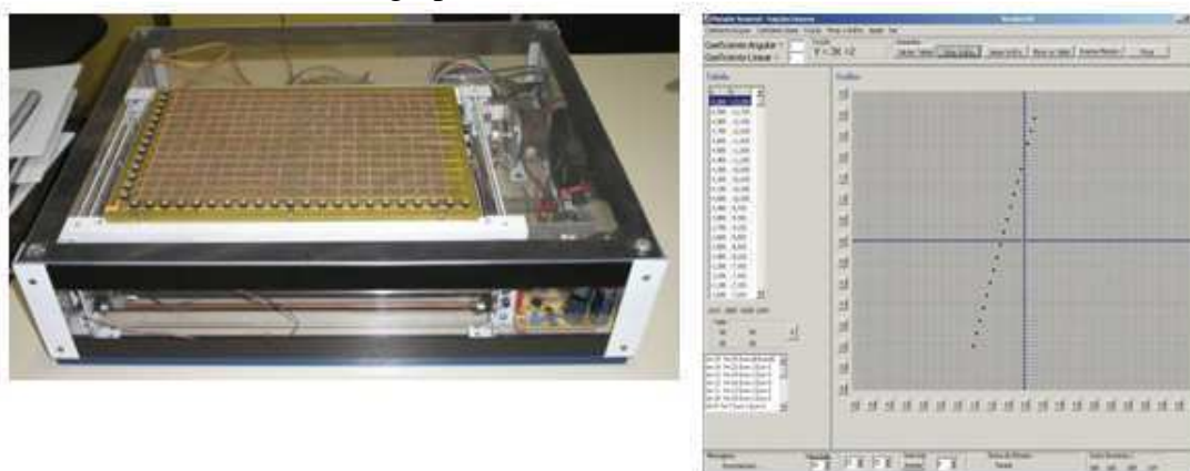
Figure 5: The current version of the tactile graphing tool and its digital interface
