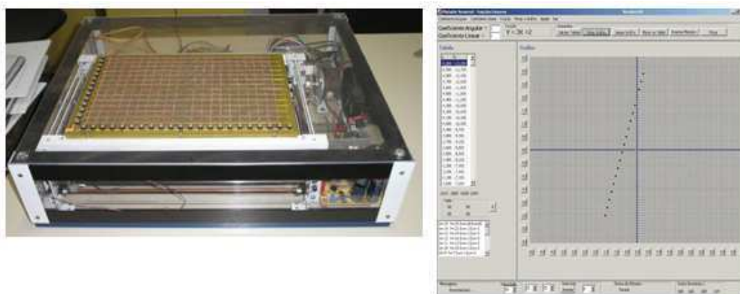
Figure 5: The current version of the tactile graphing tool and its digital interface
