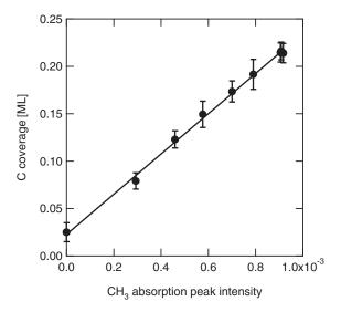
FIG. 7. Calibration of the RAIRS absorption signal CH<sub>3</sub>(ads) at 2281 cm<sup>-1</sup> in terms of C coverage on Pt(111) as determined by AES detection. The calibration data indicate a linear relationship between RAIRS absorption signal and CH<sub>3</sub>(ads) coverage with a conversion of  $\theta$ (CH<sub>3</sub>) [ML] = 211 [ML/abs]. RAIRS + 0.025.
