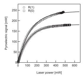
FIG. 5. Detection of vibrationally excited molecules in the molecular beam prepared by IR pumping and detected by a pyroelectric detector. The figure shows the laser power dependence of pyroelectric signal for excitation of  $CH_4(\nu_3)$  originating from the J=0 and J=1 rotational states via the R(0) and R(1) transition.
