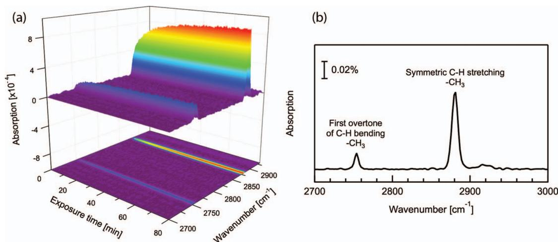
FIG. 6. RAIRS analysis of the  $\text{CH}_3(\text{ads})$  uptake on Pt(111) at  $T_s = 150$  K for an incident molecular beam of 3%  $\text{CH}_4$  in ( $E_t = 47.7$  kJ/mol,  $T_n = 700$  K): (a) Time evolution RAIRS signals during 80 min molecular beam deposition and (b) final RAIR spectrum after 80 min deposition.
