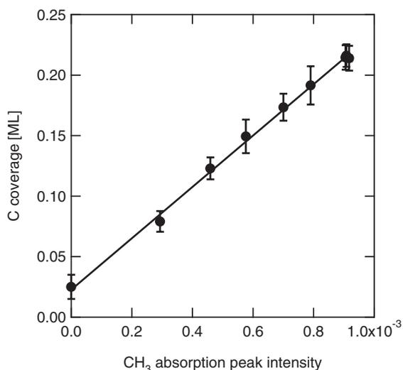
FIG. 7. Calibration of the RAIRS absorption signal  $\text{CH}_3(\text{ads})$  at  $2881\text{ cm}^{-1}$  in terms of C coverage on Pt(111) as determined by AES detection. The calibration data indicate a linear relationship between RAIRS absorption signal and  $\text{CH}_3(\text{ads})$  coverage with a conversion of  $\theta(\text{CH}_3)$  [ML] =  $211$  [ML/abs] · RAIRS +  $0.025$ .
