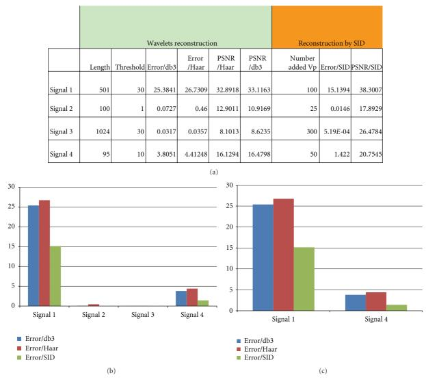
FIGURE 4: In (a): The table of comparative results showing the performance of SID. In (b): graphical representation of all the errors. In (c). The SID-based reconstruction method works better than the wavelets one.
