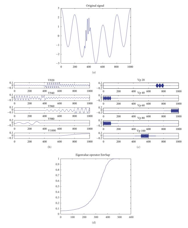
FIGURE 1: Input chirp signal in (a), some eigenvectors in (b) and all the eigenvalues for the upper envelope operator in (c). A similar result is obtained for lower envelope. Around the intermittency at the coordinate 400, each PSMF presents as nonstationarity but contributes everywhere else to the signal composition with a centred and stationary component which are Amplitude Modulation-Frequency Modulation (AM-FM). In (d) all the eigenvalues are in the segment ]0; 1] and greater than 1/17.
