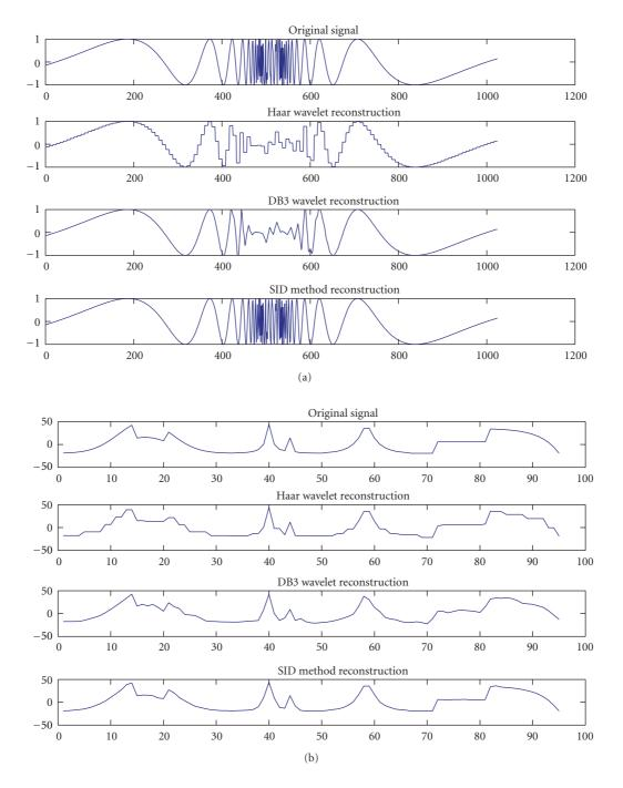
FIGURE 3: Original Signals signal 3 in (a) and signal 4 in (b), their reconstructed version by Wavelets methods and SID-based method. The SID approach works better than wavelets methods with a stronger power of reconstruction and the advantage of the skip of wavelet form choice.
