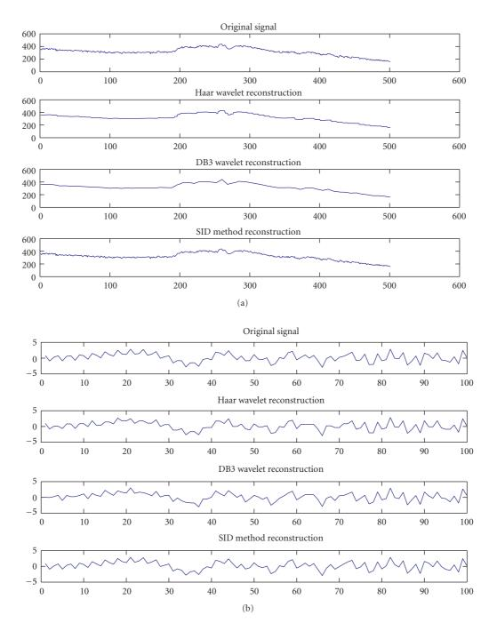
FIGURE 2: Original Signals signal 1 in (a) and signal 2 in (b), their reconstructed version by Wavelets methods and SID-based method. The SID approach works like Wavelets methods with the advantage of the skip of the choice of the mother wavelet.
