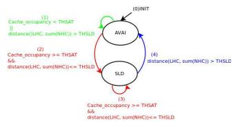
Figure 2. State machine of Data Sliding mechanism
