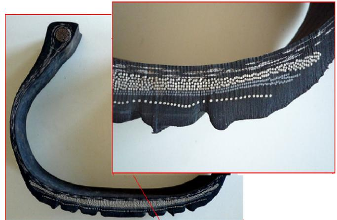
Fig. 3. Layout of the composite structure.
