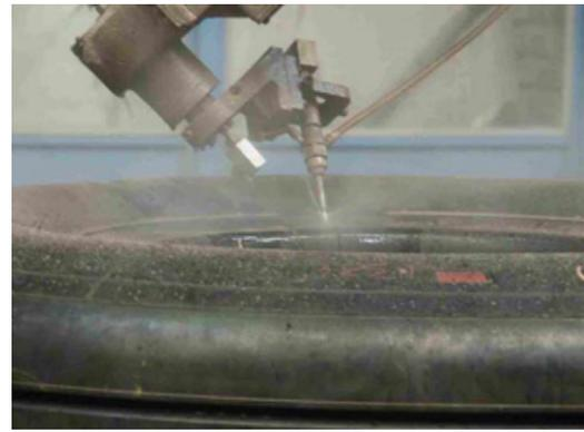
Fig. 2. Water-cutting process.
