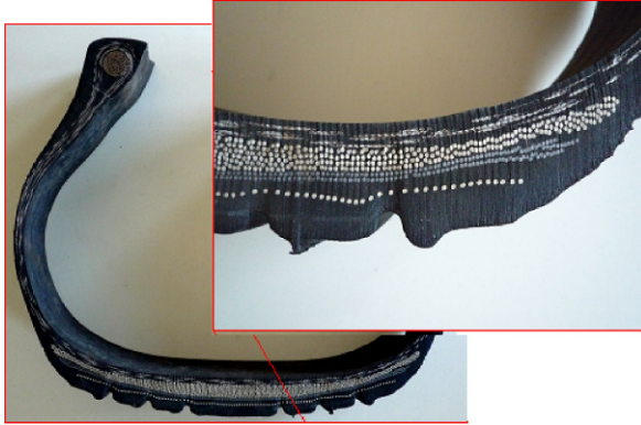
Figure 6. Water jet cutting and layout of the composite structure.
