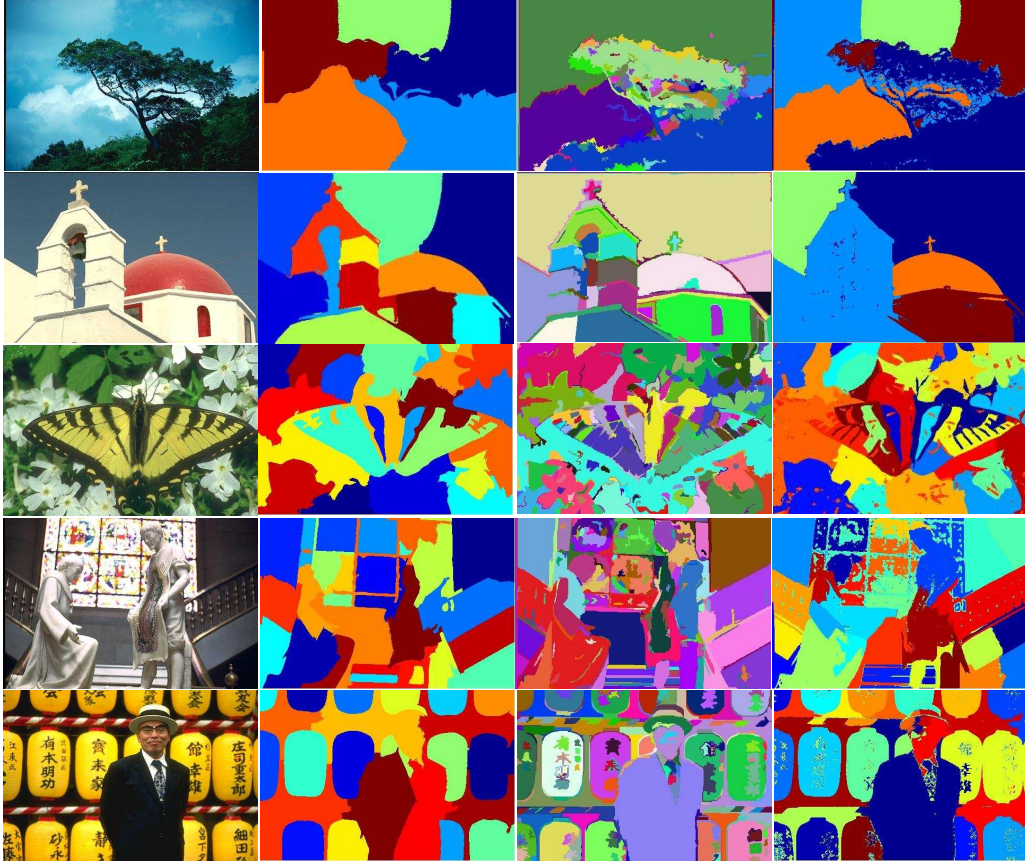
Figure 4: Visual comparison of our results with other methods on the Berkeley database (examples presented in column-wise, from left to right, are respectively the original images, NCut, GBIS and our results).
