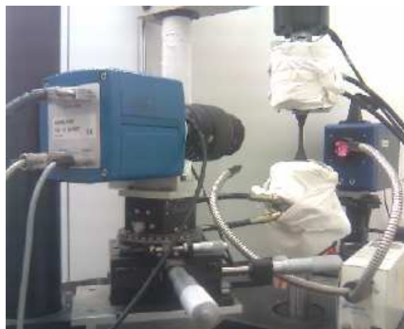
Fig. 2: Experimental arrangement. (Front): CCD camera and cold light sources, (back): IRFPA camera. The grips and columns of the testing machine are roughly wrapped to avoid parasitic reflection
