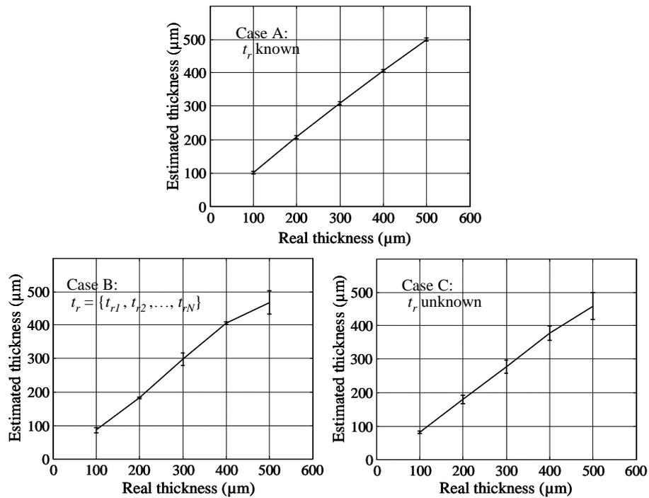
Figure 13. Results of the estimation of  $t$  obtained with experimental data featuring a 33 dB SNR. Cases  $t_r$  is known (case A), case  $t_r \in (1,5 \text{ mm}, 2 \text{ mm}, 2.5 \text{ mm}, 3 \text{ mm}, 3.5 \text{ mm})$  (case B), and case  $t_r$  is unknown (case C). In every case, the actual rib thickness value is 1.5 mm.
