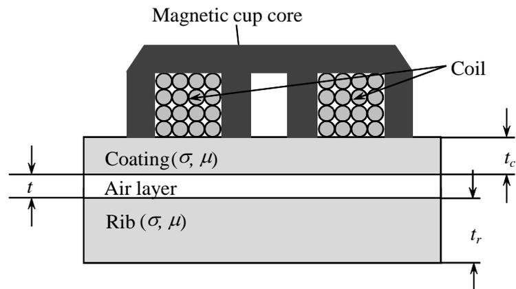
Figure 2. Eddy current cup core coil sensor placed on the inspected multilayered assembly.
