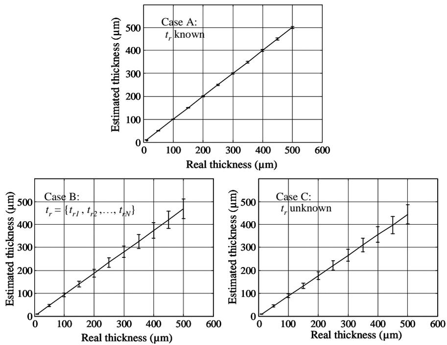
Figure 12. Results of the estimation of  $t$  obtained with simulated data featuring a 33 dB SNR. Cases  $t_r$  is known (case A), case  $t_r \in (1,5 \text{ mm}, 2 \text{ mm}, 2.5 \text{ mm}, 3 \text{ mm}, 3.5 \text{ mm})$  (case B), and case  $t_r$  is unknown (case C). In every case, the actual rib thickness value is 1.5 mm.
