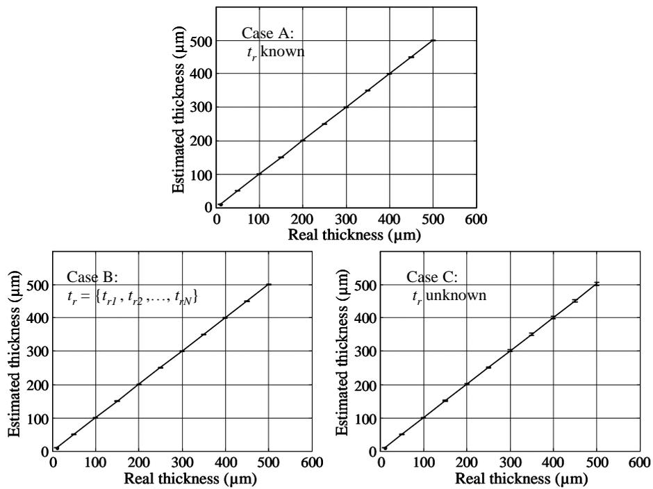
Figure 11. Results of the estimation of  $t$  obtained with simulated data featuring a 60 dB SNR. Cases  $t_r$  is known (case A), case  $t_r \in (1,5 \text{ mm}, 2 \text{ mm}, 2.5 \text{ mm}, 3 \text{ mm}, 3.5 \text{ mm})$  (case B), and case  $t_r$  is unknown (case C). In every case, the actual rib thickness value is 1.5 mm.
