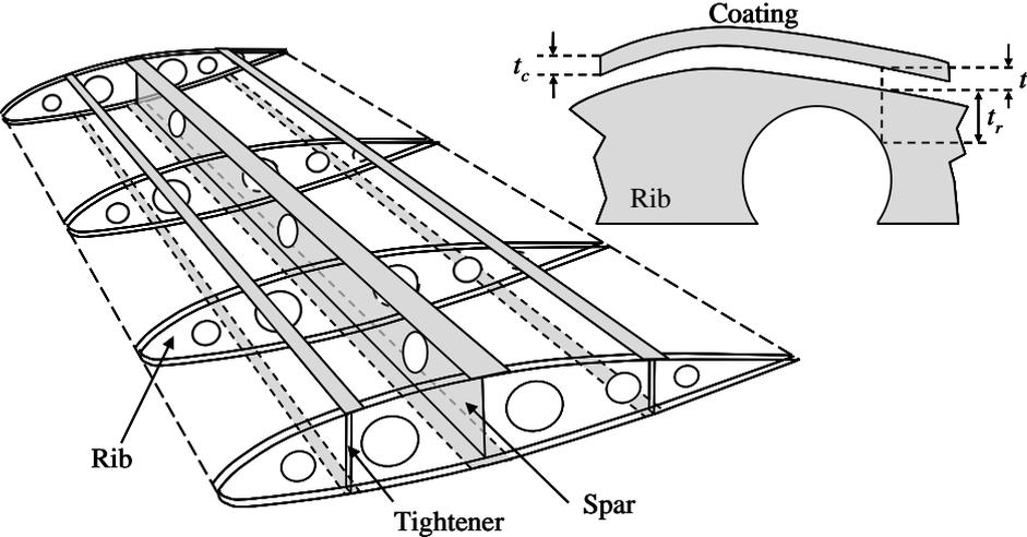
Figure 1. Structure of an aircraft wing and cut view of the assembly of a coating on a rib.
