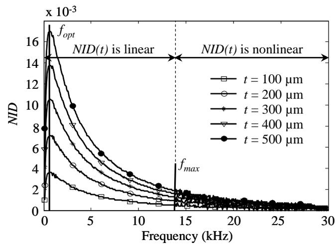
Figure 5. Variations of NID as a function of the excitation frequency  $f$ . The curves are parameterized by the air-gap  $t \in \{100 \mu\text{m}, 200 \mu\text{m}, 300 \mu\text{m}, 400 \mu\text{m}, 500 \mu\text{m}\}$ .
