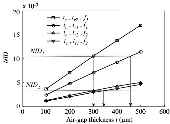
Figure 9. Set of two couples of linear characteristics  $NID(t)$ , used for the bi-frequency ( $f_1 = 680\text{Hz}$ ,  $f_2 = 6.6\text{ kHz}$ ) evaluation of  $t$ ,  $t_c$  being known and equal to 1.5 mm and  $t_r$  being unknown but possibly equal to  $t_{r1} = 1.5\text{ mm}$  or  $t_{r2} = 25\text{ mm}$ .
