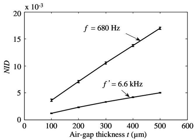
Figure 6. Linear relationship between NID and spacing  $t$  implemented at two excited frequencies, where  $t_c = t_r = 1.5 \text{ mm}$ . The error bars correspond to a confidence interval of 95%, estimated from a set of 12 measurements.
