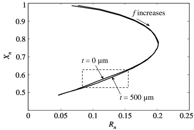
Figure 3. Universal impedance diagrams of the normalized impedance  $Z_{nt}$  of the EC sensor placed on aluminium layers assemblies and measured in the [80 Hz - 30 kHz] frequency range. The coating and the rib layers thicknesses are  $t_c = 1.5$  mm and  $t_r = 25$  mm respectively. The two measurements depicted correspond to the air-gaps  $t = 0$  and  $t = 500$   $\mu\text{m}$ .
