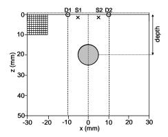
Fig. 3. Numerical 2D phantom and probe (crosses: sources "S", circles: detectors "D", large grey disc: absorption inclusion). The mesh is represented only in 1 cm<sup>2</sup>. Only the couples S1D2 and S2D1 are used for the analysis.
