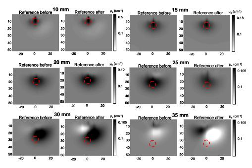
Fig. 13. Reconstructed images at iteration 15 for all depths of the inclusion, for 2 different references. From 10 to 20 mm, the reconstructed images are similar for both references. From 25 mm to deeper, analogous reconstructions obtained with the 2 different references differ very much: they are driven by photonic noise.
