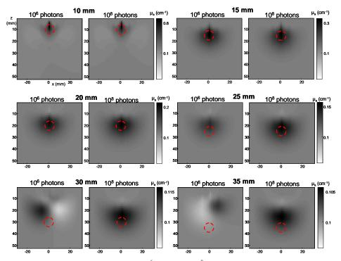
Fig. 7. Reconstructed images of  $\mu_a$  for  $10^6$  photons and  $10^8$  photons (one noise realization). The red dotted circle depicts the true position and size of the absorbing inclusion.
