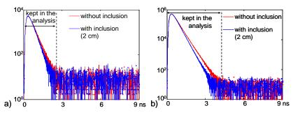
Fig. 4. Simulated signals without the inclusion (red) and with the inclusion at 2 cm depth (blue), a)  $10^6$  photons after DCR correction, b)  $10^8$  photons after DCR correction. For all: 1 noise realization only.
