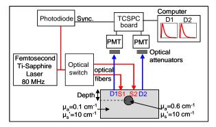
Fig. 9. TCSPC setup, probe and optical phantom.
