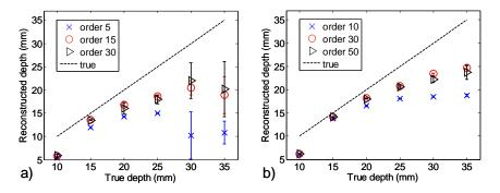
Fig. 6. Reconstructed depth versus true depth for different choices of maximum orders of MLT included for the reconstruction, a)  $10^6$  photons, b)  $10^8$  photons (error bars obtained from the 10 noise realizations).
