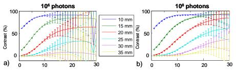
Fig. 5. Contrast on MLT orders ( $p = 3 \text{ ns}^{-1}$ ) for the different depths for S1D2, a) 10<sup>6</sup> photons, b) 10<sup>8</sup> photons (error bars are obtained from the 10 noise realizations).
