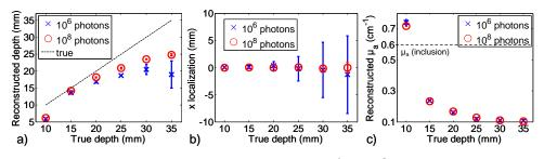
Fig. 8. Summarized reconstruction performances for  $10^6$  and  $10^8$  photons for 10 noise realizations, a) reconstructed depth, b) x localization, c) Mean reconstructed  $\mu_a$ .
