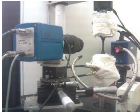
Fig. 2. Experimental set-up: (front): CCD camera and cold light sources, (back): IRFPA camera. The grips and columns of the testing machine are roughly wrapped to avoid parasitic reflection interference.
