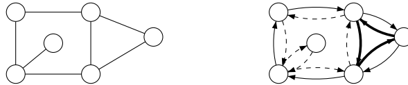
Figure 26: Any edge is met twice, thus composed of two arcs (represented with different line styles), when used to describe the faces of a plane graph.
