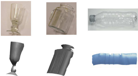
Figure 4 – 3D Digitization results obtained by SFH on transparent surfaces
