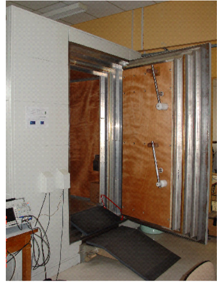
Figure 6. View of the GREYC laboratory magnetically shielded room (composed of six layers: 1 in soft iron, 4 in \mu -metal, 1 in aluminum).
