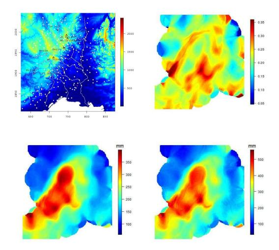
Figure 3: Upper left: map of the Cévennes-Vivarais region, horizontally: longitude (km), vertically: latitude (km), the color scale represents the altitude (m), the white dots represent some raingauge stations, upper right:  $\hat{\gamma}_n(x)$ , bottom left:  $\widehat{RVaR}_n^W(\beta_n|x)$  for a 100-year return period, bottom right:  $\widehat{RCTE}_n^W(\beta_n|x)$  for a 100-year return period.
