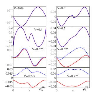
FIG. 3: (color online) Current-phase relations  $I_a(\varphi_b^{(0)})$  (red, full curve) and  $I_b(\varphi_b^{(0)})$  (blue, dashed curve), in units of  $e\Delta/\hbar$ , in the quartet configuration  $V_a = -V_b$ , for the resonant dots regime:  $\varepsilon_a = -\varepsilon_b = 0.4\Delta$  and  $\Gamma = 0.1\Delta$ . Note the different y scales in the different panels.
