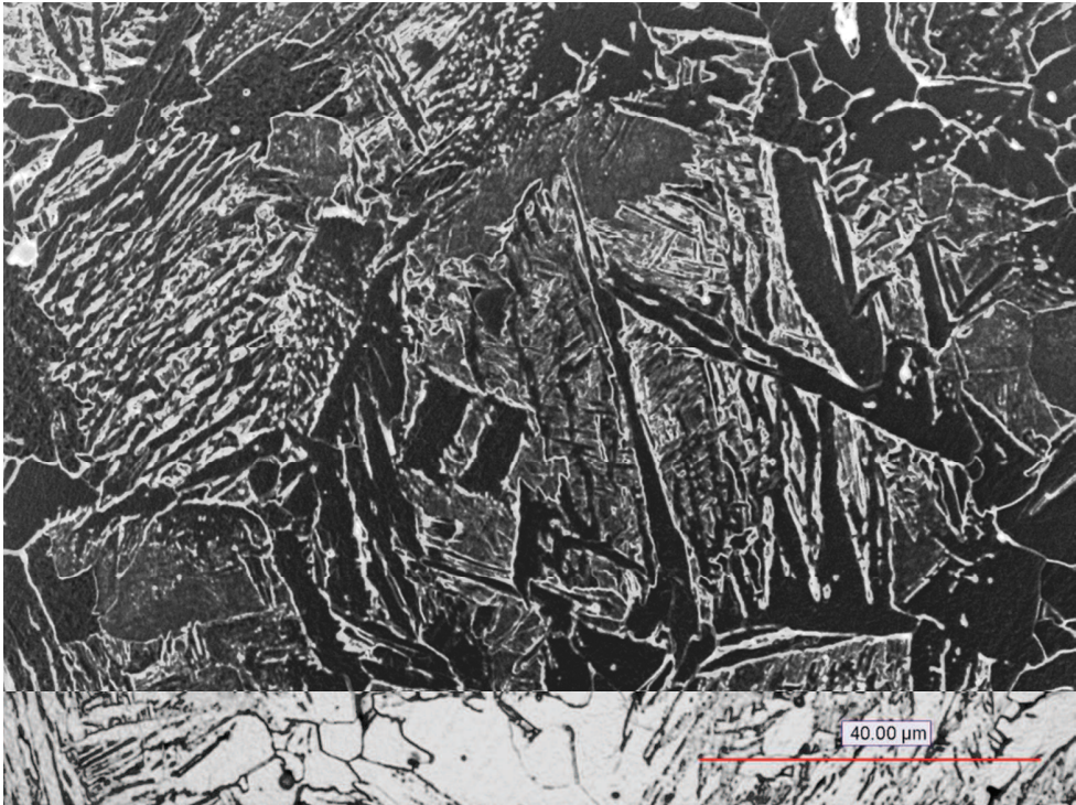
FIG. 10: microstructure of the carbonitrided C18 steel. (a) : Microstructure of the substrate (b) : Microstructure of the surface
