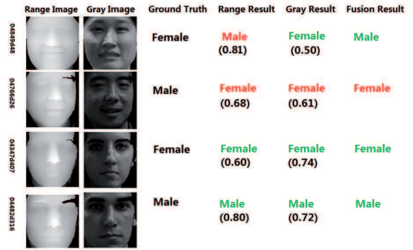
Fig. 6. Fusion with results from range and gray images. For each subject, from left to right, the columns are: the pre-processed range image, the preprocessed gray image, the ground truth of gender, the predicted class label and the probability with range image, the predicted class label and the probability with gray image, the predicted class label of fusion.
