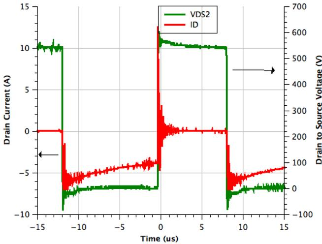
Fig. 8. Drain-to-source voltage and drain current in the low side device for a input voltage of 540 V at 50 kHz with a load current of 5 A
