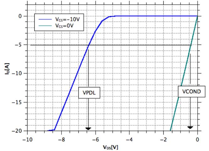
Fig. 6. Reverse static characterizations of a VJFET. For  $I_D = -5 A$  and  $V_{GS} = -10 V$ ,  $V_{PDL} \approx -6.5 V$ . For  $I_D = -5 A$  and  $V_{GS} = 0 V$ ,  $V_{COND} \approx -400 mV$ .
