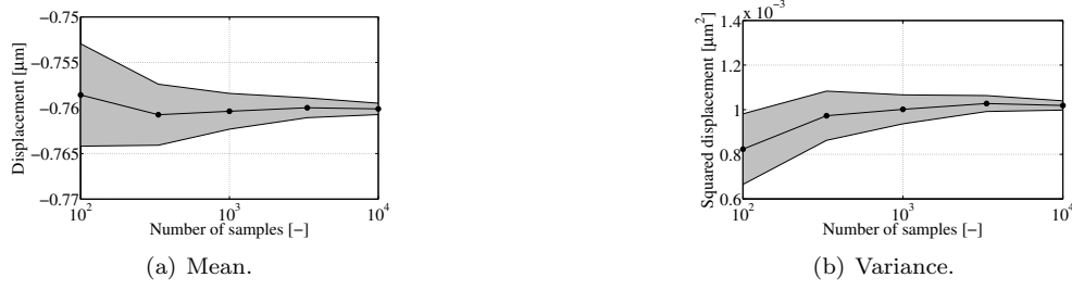
FIG. 5.9. Convergence study: (a) sample average (circles) and 95% confidence region for the mean (filled) and (b) sample variance (circles) and 95% confidence region for the variance (filled) of the vertical component of the displacement at the mid point ( x_1 = 70 \mu\text{m} , x_2 = 4.25 \mu\text{m} ) for \epsilon_1 = 2.5 \times 10^{-3} and \epsilon_2 = 1 \times 10^{-8} as a function of the number of samples.
