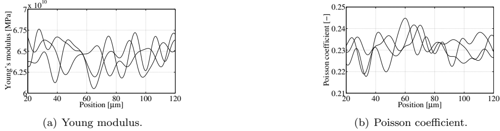
FIG. 5.3. Stochastic coupled problem: a few samples of (a) the random Young modulus field and (b) the random Poisson coefficient field as a function of the horizontal position, that is, as a function of x_1 , at the vertical position of the neutral fiber, that is, at x_2 = 4.25 \mu\text{m} .
