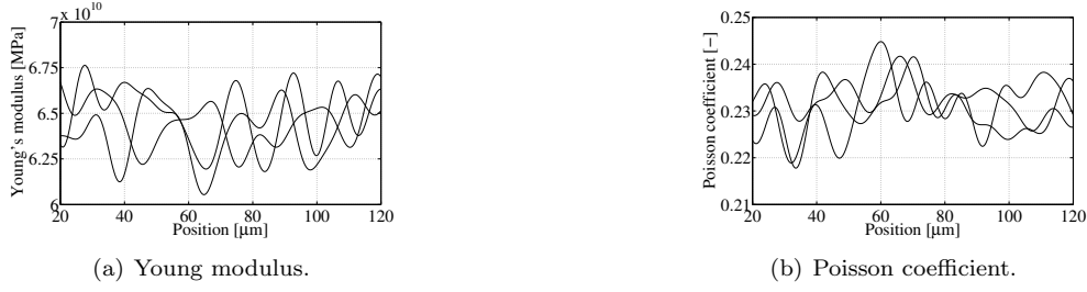
FIG. 5.3. Stochastic coupled problem: a few samples of (a) the random Young modulus field and (b) the random Poisson coefficient field as a function of the horizontal position, that is, as a function of x_1 , at the vertical position of the neutral fiber, that is, at x_2 = 4.25 \mu\text{m} .
